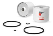
Largest OD88.00 mmLargest End ID38.00 mmLength72.00 mmEfficiency Test StdISO 19438Rated Flow0.9 L/mElement Collapse/Burst, Min400 kPa
