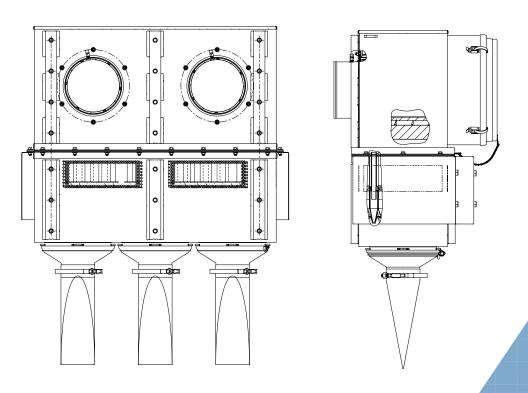
The SSG air cleaner series is a family of two-stage RadialSeal™ engine air cleaners that provide improved reliability and better durability compared to axial seal style air cleaner designs.
