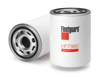
180.00 mm Length Largest OD 128.00 mm Thread Form British **BPV OPENING DP** No **Gasket Inside Diameter** 98.00 mm **Gasket OD** 107.00 mm **Hydrostatic Burst Minimum** 1500 kPa Particle Size at Beta 75 12 micron Internal Thread Type Flow Direction Outside In
