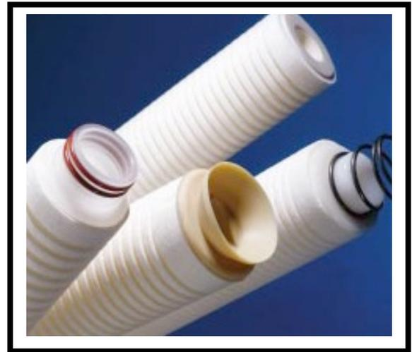
All PCB cartridges are designed to yield high particle capture even under pulsating flow. Each grade is benchmarked to yield consistency in terms of end filtrate quality throughout the life of the filter. Available in a range of ratings from 0.5 to 100 µm, PCB filters are available in a range of lengths & end Treatment options including various DOE & SOE, configurations.
